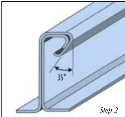
All panels are also punched at the factory for precise alignment. Moveable clips allow for up to 2" of movement in either direction to allow for expansion and contraction of the roof. Panels are available in 22 and 24 gage and feature the Butler-Cote finish system for protection, available in an array of colors to give designers and building owners great latitude with design decisions.
