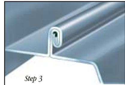
**360 degree 3-stage "Pittsburgh" double lock seam**
